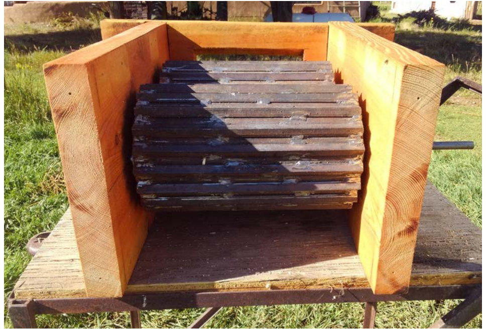
Roller placement between side panels
