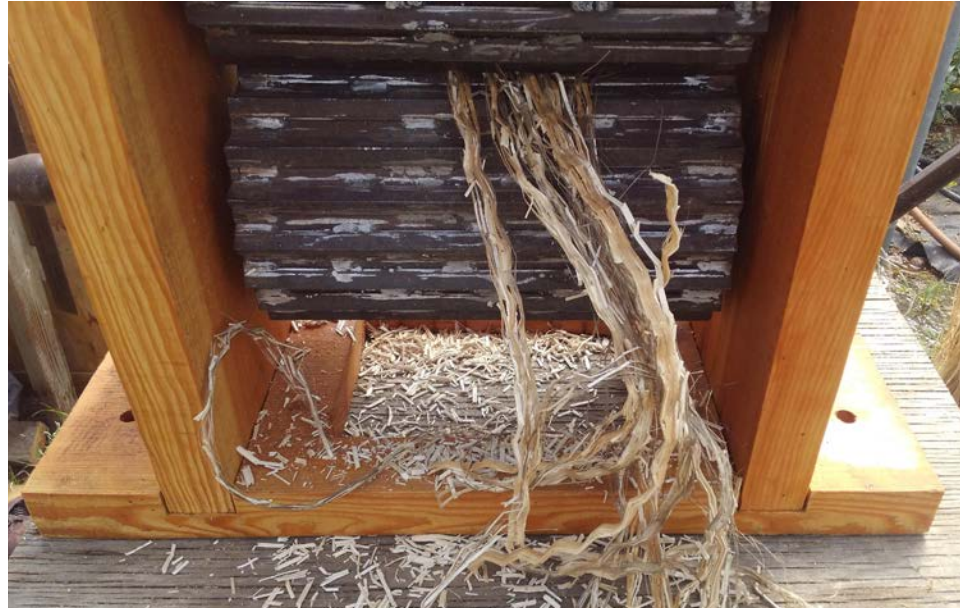
Left to right: Operation of Steel Roller Hemp Break, close up of crimped hemp stalks and shiv pieces
