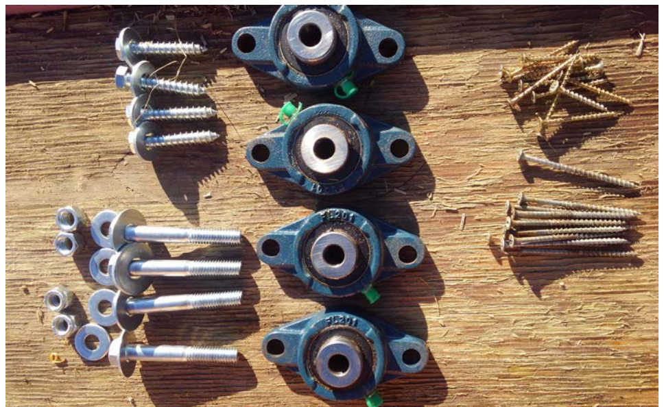
Bearing blocks, bolts and deck screws
