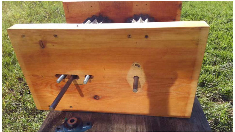
Side view of side panel showing roller shafts
