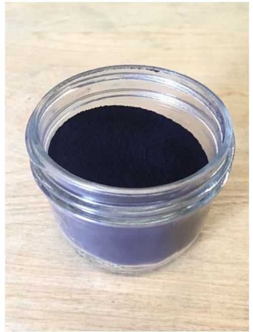
In True Blue's trials, approximately 90 lbs of plant material was processed in 100-gallon tanks, producing pigment of 22% purity at a pure indigo yield of 0.06% of fresh plant weight. (Photos by Nicholas Wenner)
