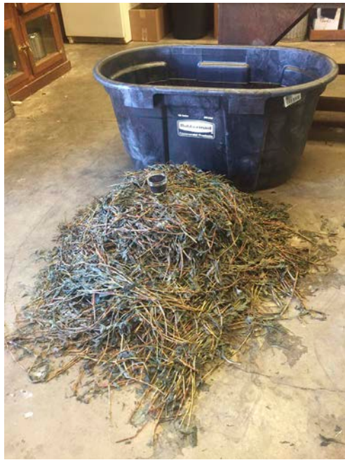
In True Blue's trials, approximately 90 lbs of plant material was processed in 100-gallon tanks, producing pigment of 22% purity at a pure indigo yield of 0.06% of fresh plant weight. (Photos by Nicholas Wenner)
