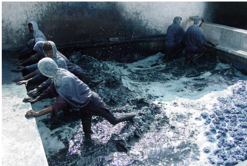
(Above) Indian workers oxidizing a tank of indigo 49 (Below) Diagram showing the operation of a filter press 50
