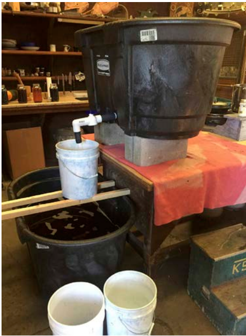
In True Blue's trials, approximately 90 lbs of plant material was processed in 100-gallon tanks, producing pigment of 22% purity at a pure indigo yield of 0.06% of fresh plant weight. (Photos by Nicholas Wenner)
