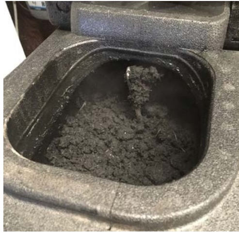
Left: crushed, sifted, and rehydrated indigo leaves in a benchtop composter; center: the same leaves after 1 week of composting. The machine's rotating stirring bar can be seen in the second photo. Right: using industrial composting machines, indigo compost can be made in 3-4 weeks with minimal labor. (Photos by Nicholas Wenner)
