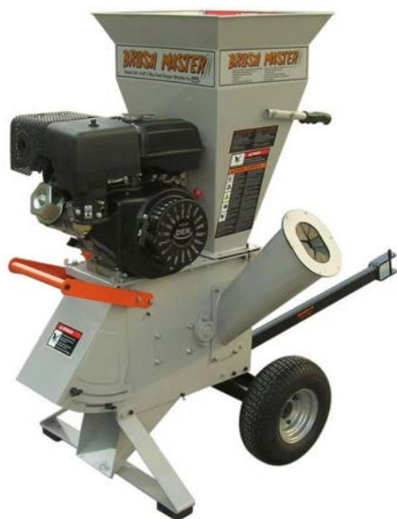
A gas-powered chipper for cutting up indigo for the winnowing step 97
