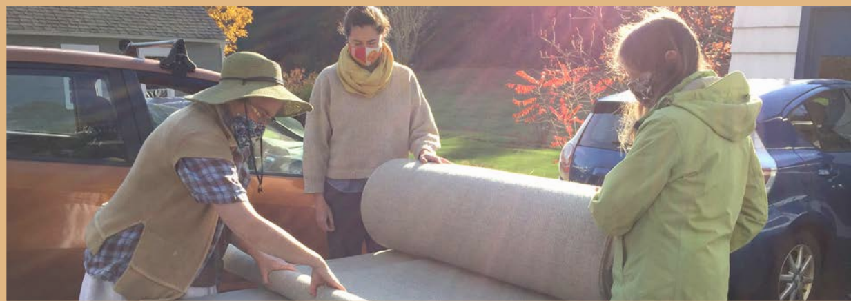
More than one pattern can be woven on the same warp, then we cut apart and re-roll each section (Gretchen Laise, Katie Cavacco, Peggy Hart).
