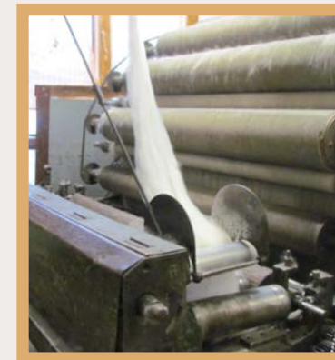
Carding machine at Green Mountain Spinnery Putney, VT. Green Mountain Spinnery uses a woolen spinning system.
