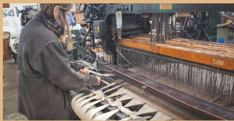
Peggy Hart of Bedfellows Blankets, Shelburne Falls, MA. The warp is wound with single yarns, threads are drawn through the heddles, and the warp is tied onto the loom before weaving.
