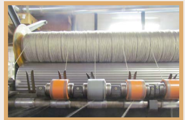
Pencil roving ready to add twist at Green Mountain Spinnery. After the fiber is washed, picked, and carded, it is divided into thin sections before twist is added to create the yarns.
